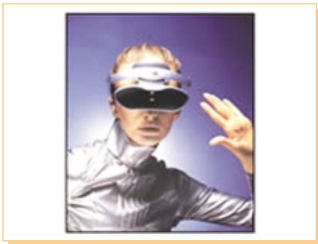
Image 3. Head Mounted Display device
